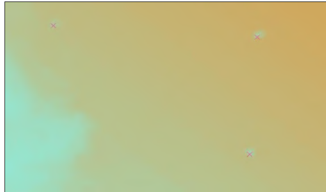
Figure 10 Section of DEM indicating the impact of Shipwrecks in the Source Data (a cross indicates a shipwreck)
